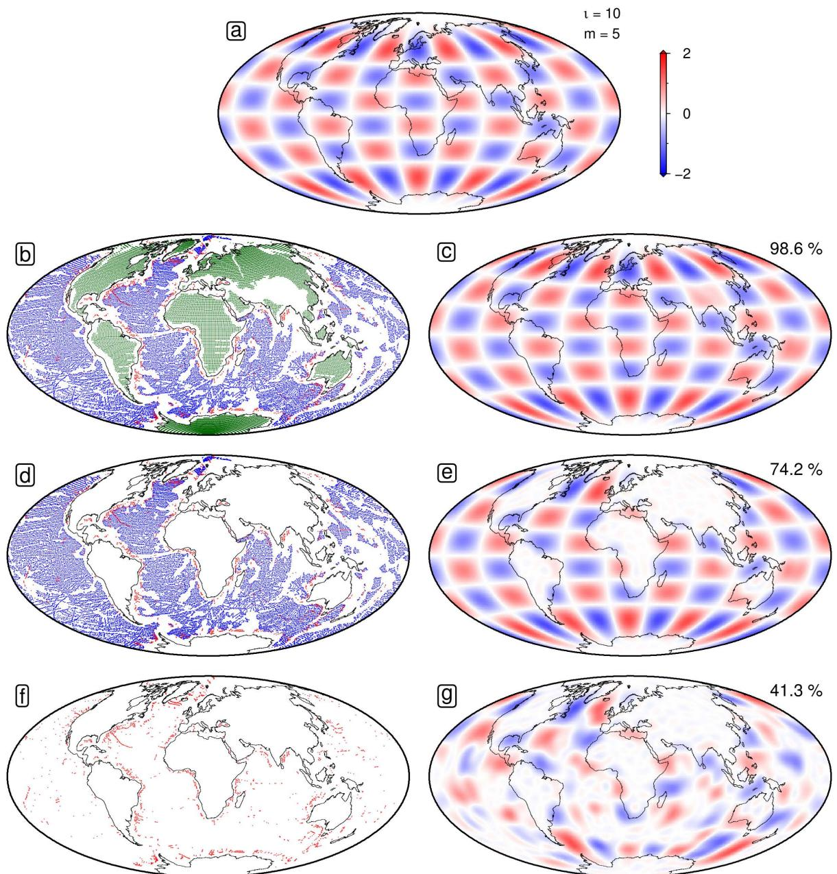
**Figure S5: Synthetic checkerboard test.** (a) Input spherical harmonic function with  $l = 10$  and  $m = 5$ . (b) Locations of all oceanic and continental data points used to sub-sample input model. (c) Resulting spherical harmonic fit with recovery of input coefficients. (d) All measurements from oceanic realm alone. (e) Recovery obtained using (d). (f) Only spot measurements from oceanic realm (symbols from Figure 1b of main text). (g) Recovery obtained using (f).
