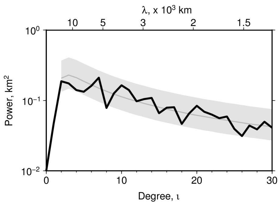
**Figure S10: Kaula's rule.** Solid line = power spectrum of observational database (Figure 5b in main text); grey line/band = power spectrum calculated using Equation 4 for  $Z = 12 \pm 3 \text{ mGal km}^{-1}$ .
