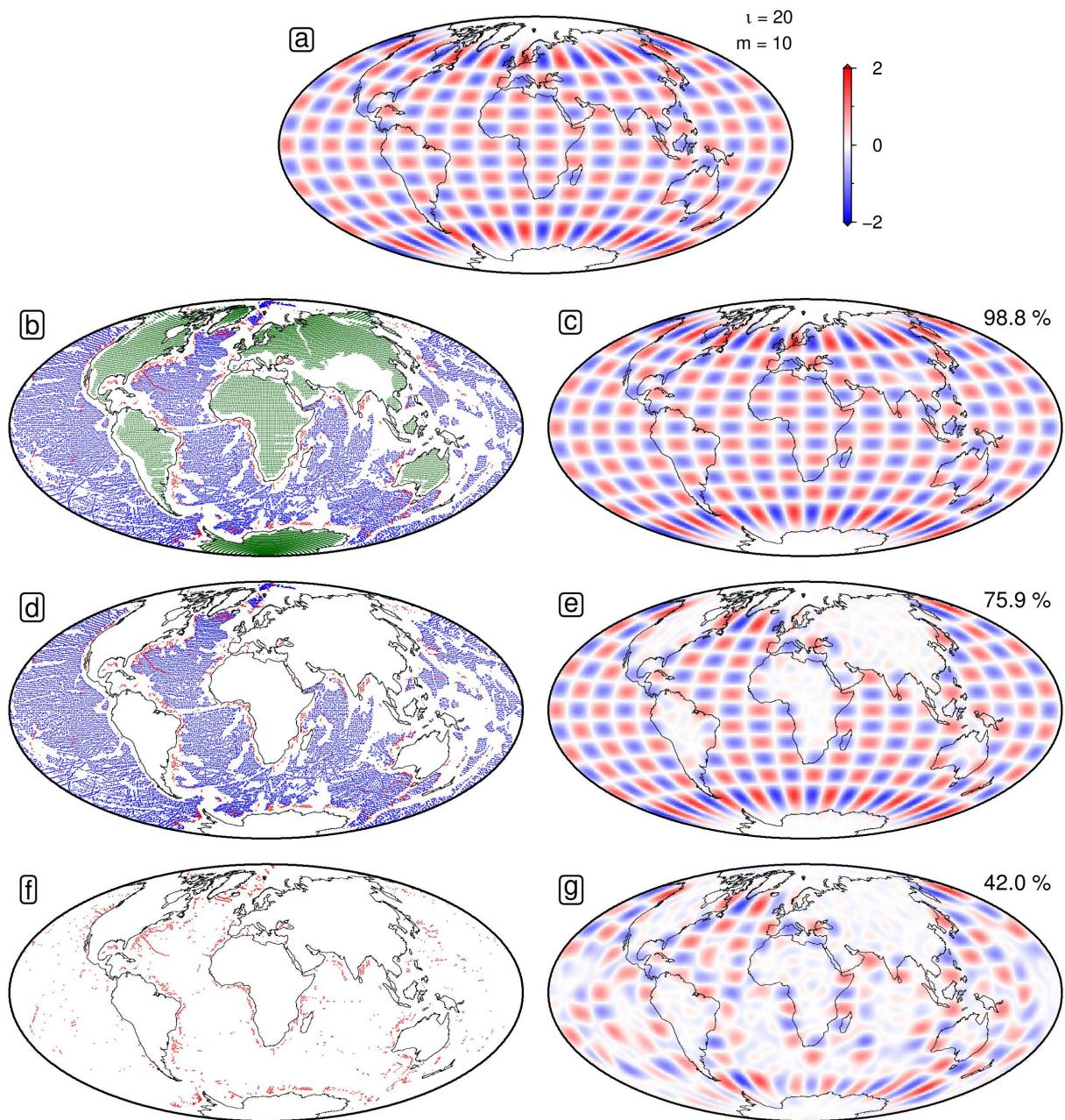
**Figure S6: Synthetic checkerboard test.** (a) Input spherical harmonic function with  $l = 20$  and  $m = 10$ . (b) Locations of all oceanic and continental data points used to sub-sample input model. (c) Resulting spherical harmonic fit with recovery of input coefficients. (d) All measurements from oceanic realm alone. (e) Recovery obtained using (d). (f) Only spot measurements from oceanic realm (symbols from Figure 1b of main text). (g) Recovery obtained using (f).
