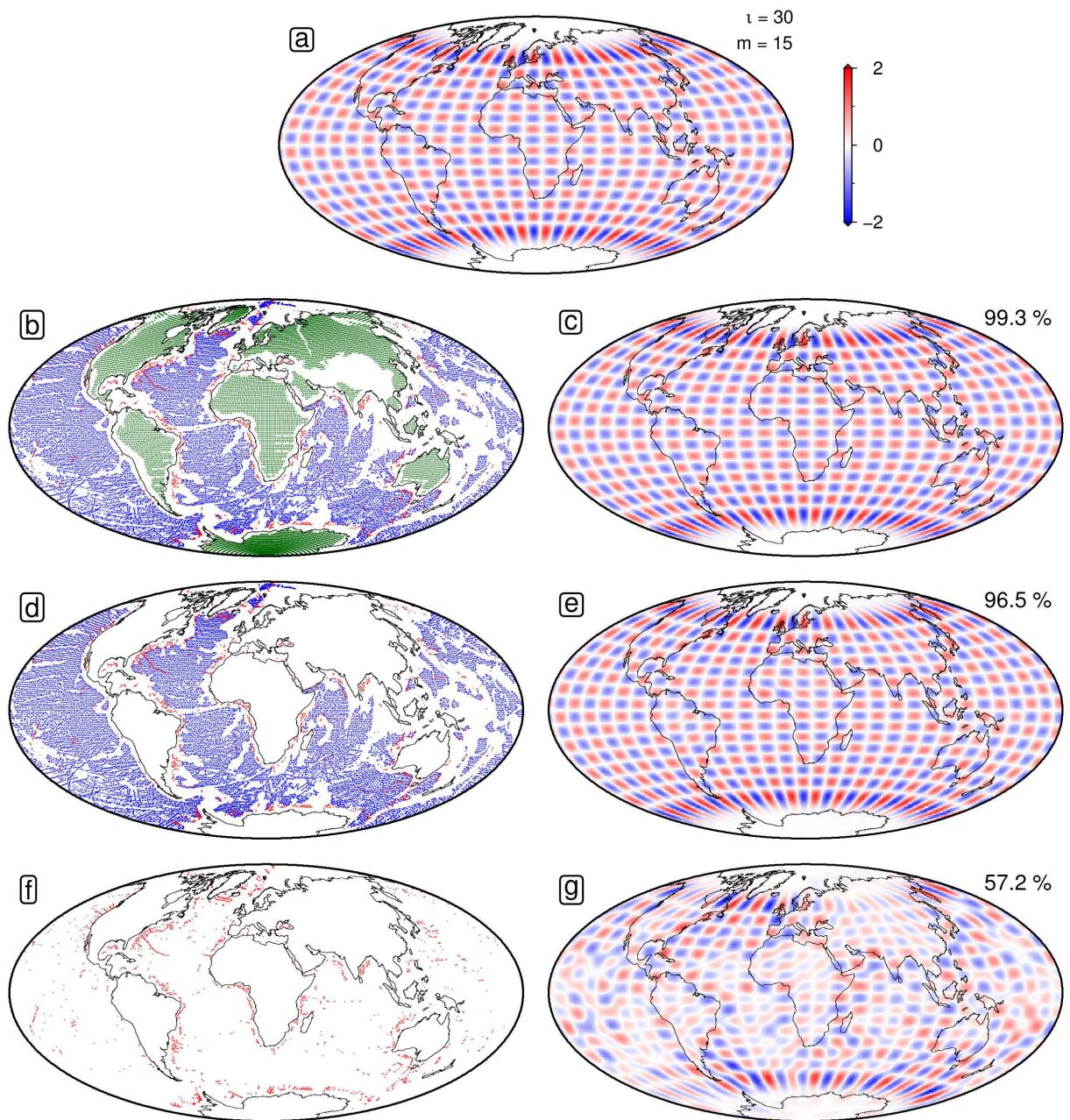
**Figure S7: Synthetic checkerboard test.** (a) Input spherical harmonic function with  $l = 30$  and  $m = 15$ . (b) Locations of all oceanic and continental data points used to sub-sample input model. (c) Resulting spherical harmonic fit with recovery of input coefficients. (d) All measurements from oceanic realm alone. (e) Recovery obtained using (d). (f) Only spot measurements from oceanic realm (symbols from Figure 1b of main text). (g) Recovery obtained using (f).
